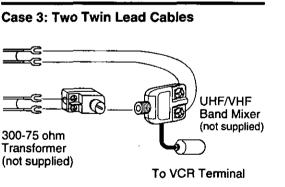
If your TV has both post and plug-type VHF • terminals, the post connection is recommended to minimize signal loss.
