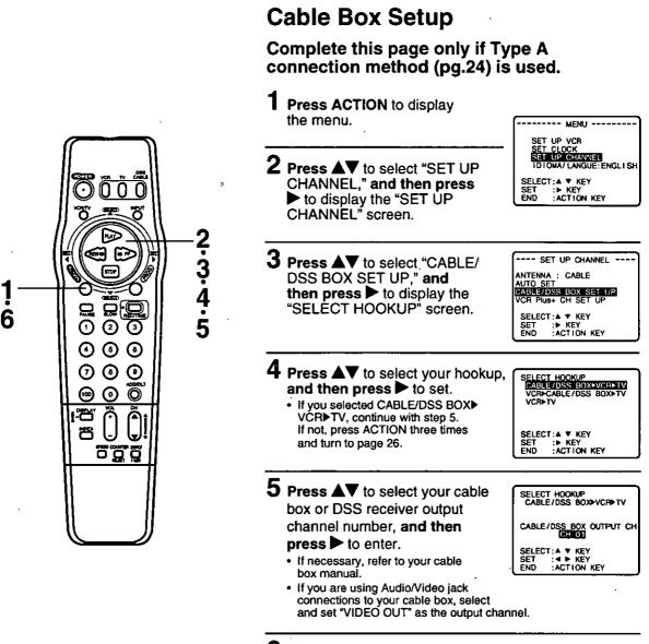
**6** Press ACTION twice to end the setup and return to the normal screen.
